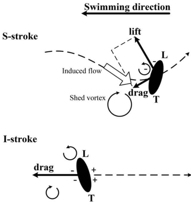
**Figure 8** — Schematic of the findings of Matsuuchi et al<sup>44</sup> and Takagi et al.<sup>43</sup> L indicates the little finger side, T the thumb side of the hand.
