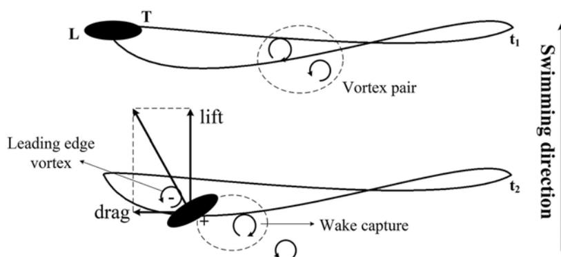
**Figure 7** — Schematic of the findings of Takagi et al.<sup>42</sup> L indicates the little finger side, T the thumb side of the hand.
