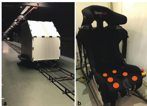
Fig. 1 a The linear sled that was used in this study. The illuminated cabin offered an enclosed space that removed external visual and air-flow cues. b Interior view of the cabin where the participants were seated. The stationary visual frame of reference provided by the cabin resembles the context of a car ride without looking outside. A printed version of the used motion sickness scale was taped onto the wall in front of the participants. Participants could also see a webcam which was used for observation. The rally seat offered a head rest and a five-point seat belt for safety. The orange dots indicate the position of the six vibrotactile actuators
